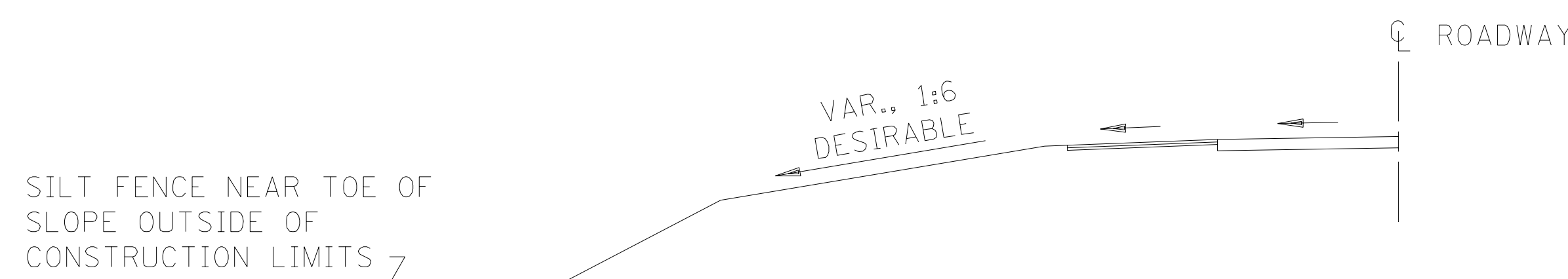
LOCATION OF SILT FENCE FOR PEREMITER CONTROL
