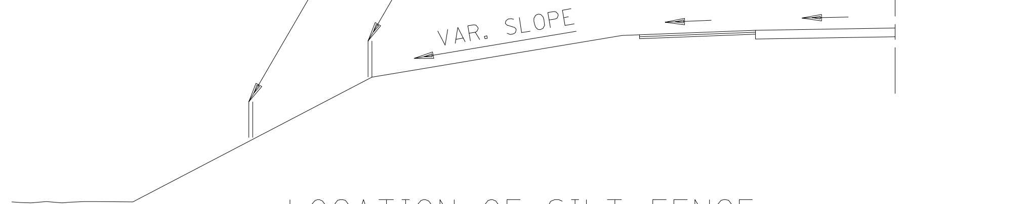
LOCATION OF SILT FENCE FOR SEDIMENT CONTROL
